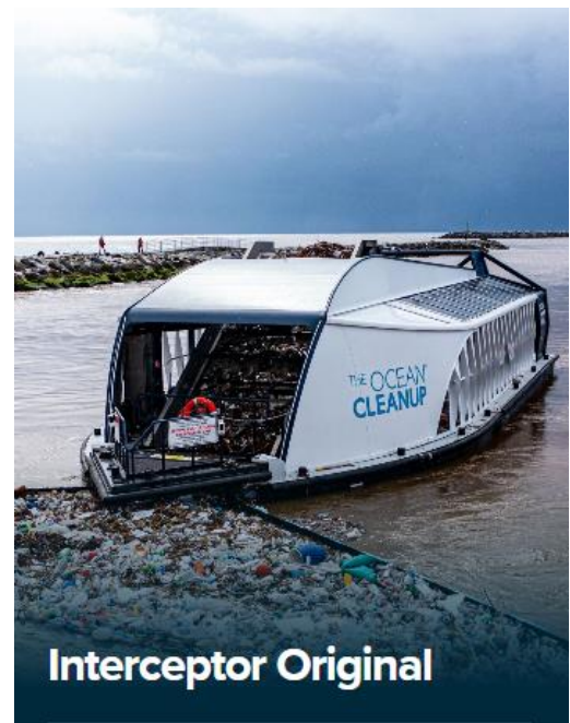
Figure 4 (right) – The Original Interceptor used on The Ocean Cleanup's first ever river cleanup, featuring solar powered mechanics, smart processing. Being autonomous with a large cleaning capacity, it is the main technology they used to evaluate for the feasibility in any new river project.
